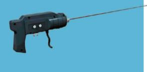
This SS 316 high temperature probe includes a 2.5 meter cable and is intended for measuring the temperature of the combustion air available with different length as user required. This means that youcan accurately measure temperatures and combustion efficiency in central heating systems where the combustion air is supplied via a separate channel.21
